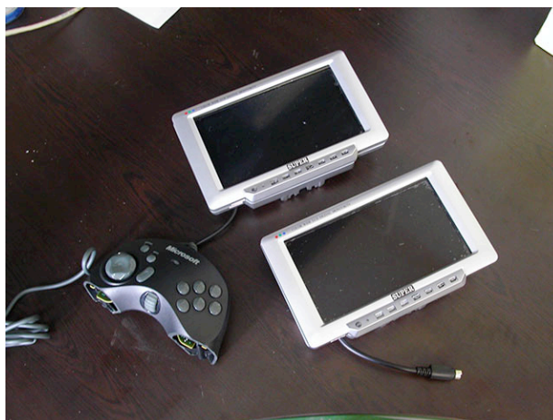
Basic Components: 2 7-inch TV panels and an old PC game controller.
