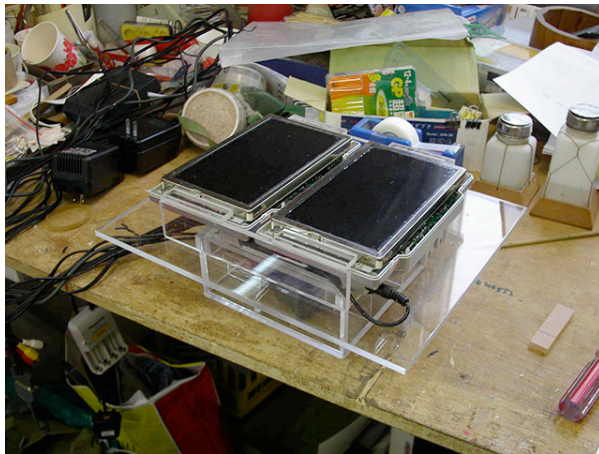
The TV panels mounted together in an acrylic frame....
