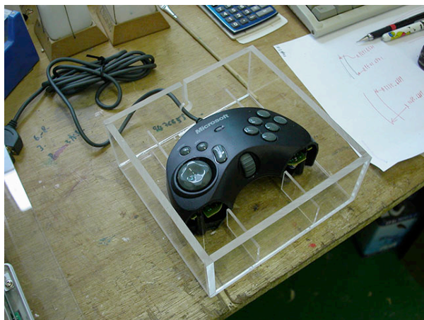
The handles of the game controller are removed and the controller mounted in an acrylic box. Most of the buttons on the controller are retained for possible future applications.
